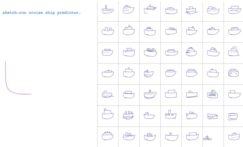
Figure 16: This figure displays an example of the predictive power of RNNs, similar to the RNN used in the World Models paper. Here a single line leads to numerous predictions of what the drawing will look like given that it should be a cruise ship. This example comes from SketchRNN, a free online game for experimenting with RNNs [30].
